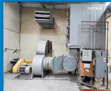
40-HP Dust Hog 16-Cartridge Dust Collector
