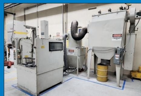
Guyson RXS900 Multi-Station Blast System w/ Dust Collector
