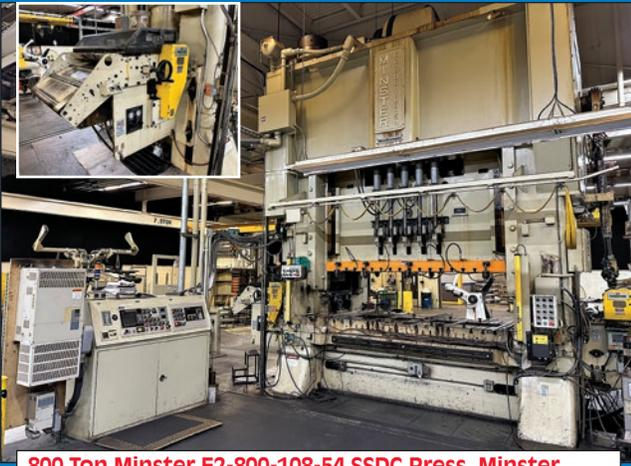
800 Ton Minster E2-800-108-54 SSDC Press, Minster Servo Feed Line
