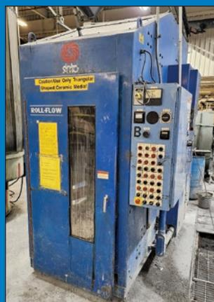
Sinto Roll-Flow EVF-08R Centrifugal Disc Finisher
